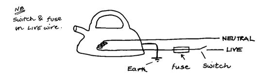
The electric current flows through the live wire, into the heating element and out through the neutral wire. The fuse and switch are placed in the live wire (see note below). The Earth wire is connected to the outside casing of the kettle. Normally, no current flows through the Earth wire, so what is it for?
