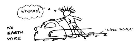
If there is a fault and a live wire touches the casing, then a person touches the casing, the electricity will go through the person and into the ground. The person could be killed.
