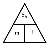
where:  $E_h$  is the heat energy absorbed or given out by an object (J) m is the mass of a material (kg)
