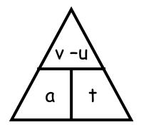
where: a is the vertical acceleration of an object  $(m/s^2)$   $v_v$  is the final vertical velocity of an object (m/s)u is the initial vertical velocity of an object (m/s)t is the time that an object accelerates for (s)
