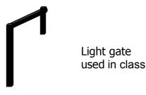
A light gate consists of a light source aimed at a photocell. The photocell is connected to an electronic timer or computer. The timer measures how long an object takes to cut the light beam. The distance travelled is the length of the object which passes through the beam. Often a card is attached so that the card passes through the beam. The length of the card is easy to measure. The instantaneous speed as the vehicle passes through the light gate is then calculated using:
