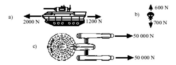
3. By using a scale diagram or otherwise, find the resultant of the following pairs of forces. Remember to draw the vectors "tip to tail".
