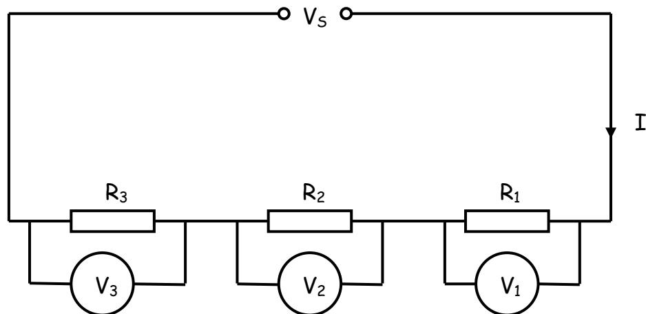
In a SERIES circuit *the current through each resistor is the same. To find the current use the formula:*
