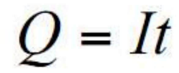
To calculate the amount of charge transferred in an electrical circuit.
