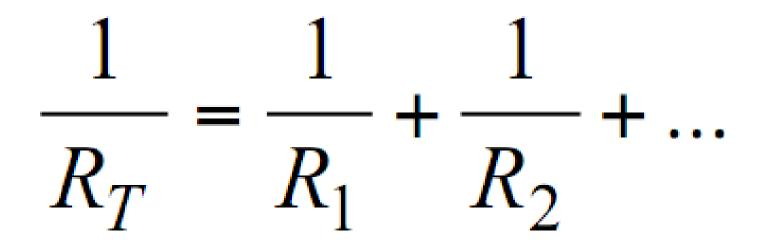
To calculate the total resistance of resistors in parallel.
