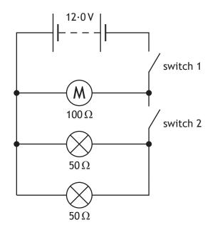
(a) Switch 1 is now closed. Calculate the power dissipated in the motor when operating. Space for working and answer
