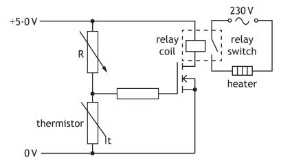
(i) Explain how the circuit operates to switch on the heater when the temperature falls below a certain value.
