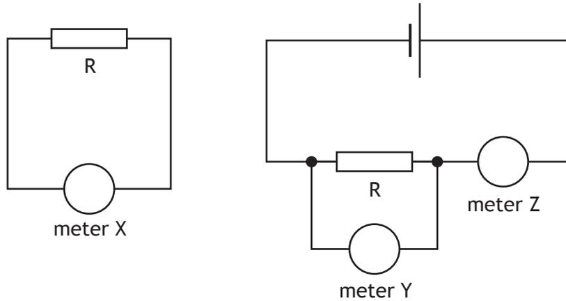
Both circuits are used to determine the resistance of resistor R.
