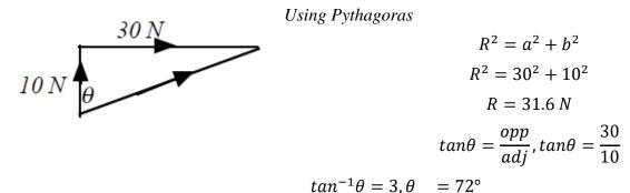
In some cases that means that the two vectors have to be redrawn so that they are being added "head to tail". See example below.
