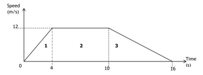
It is best to split the area under the graph into rectangles and triangles. Calculate the area of each and then add them together. [Area of a triangle is  $\frac{1}{2}$  base x height]
