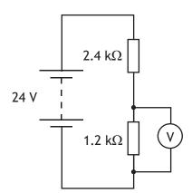
The reading on the voltmeter is
