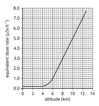
The aircraft flies at an altitude of 11 km for 3.5 hours. Calculate the equivalent dose received by a crew member during this time. Space for working and answer
